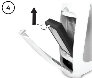
Remove the Air Filter by pulling the tab out. Then, pull the Air Filter straight up and out of the Filter Housing compartment.
