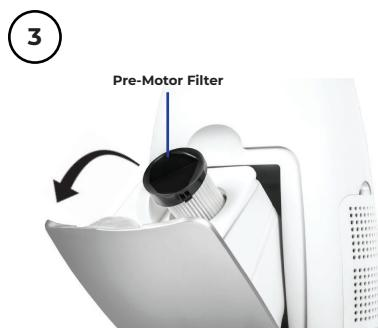
Remove the Pre-Motor Filter by grasping the Pre-Motor Filter handle and turn counter-clockwise to the unlock position. Pull Pre-Motor Filter straight up and out of the top of the Canister.
