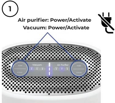
Starting with the Vacuum, touch the Power button, and cycle to the off position. On the air purifier side, touch the Power button and cycle to the off position. Then, unplug the EyeVac Air.
