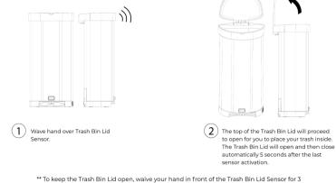
\*\* To keep the Trash Bin Lid open, waive your hand in front of the Trash Bin Lid Sensor for 3 seconds. The Trash Bin Lid will open and remain open. To close and return to normal operation, waive your hand in front of the Trash Bin Lid Sensor for 3 seconds.
