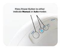
**3.** Turn Power Button on (button located on top, back of unit). Unit will be in Automatic Mode. Press Power Button again to select Manual Mode. Blue indicator light will show unit is powered on.
